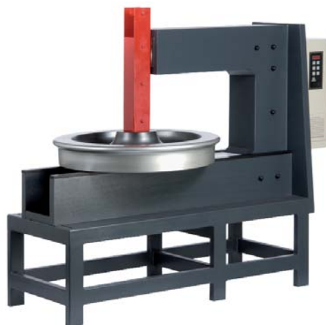
Betex GIANT heating cap. 3500 kg
